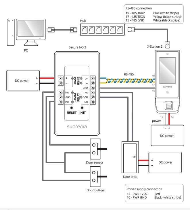
• X-Station 2 can be used as a multi-door controller with the slave devices with the RS485 cable. The slave devices are used as dummy readers and authentication is performed in the master device.
